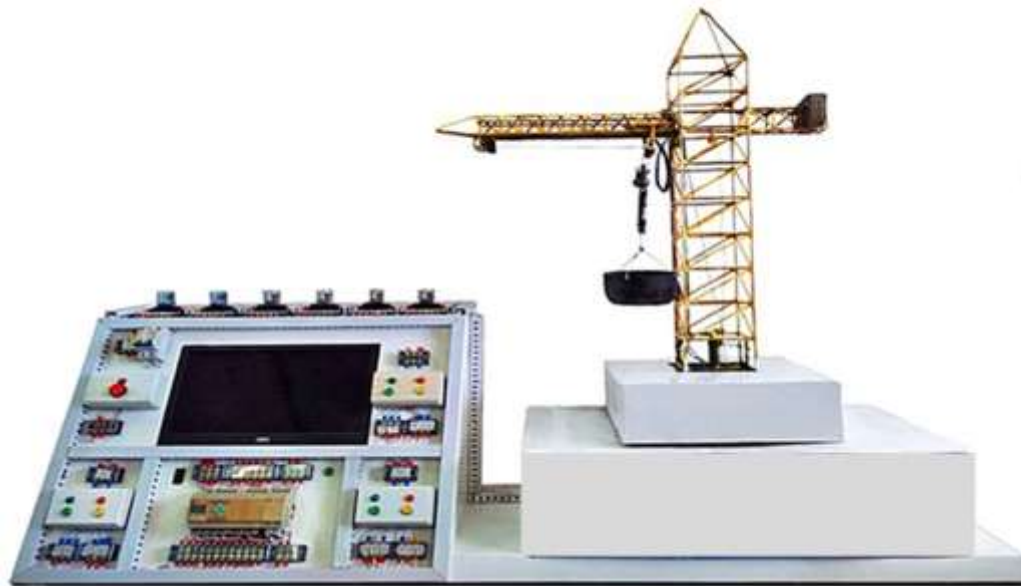
Figure 2. Perspective View of the Computer- Assisted PLC-Controlled Tower Crane System
